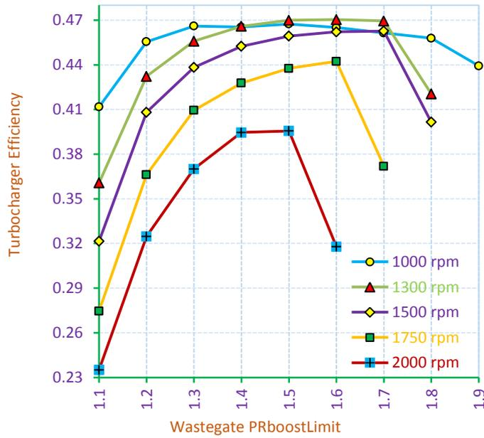
Fig10. Total Turbocharger Efficiency comparison at different speeds.
