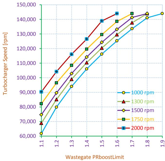
Fig11. Turbocharger speed VS. Limiting boost pressure ratio.
