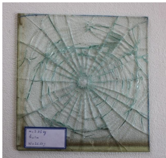
Fig14. .specimen after test code D-B-T-6
