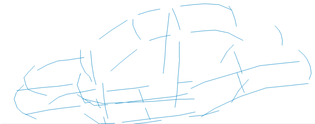
Fig3.: Equivalent beam modeling of the BIW
