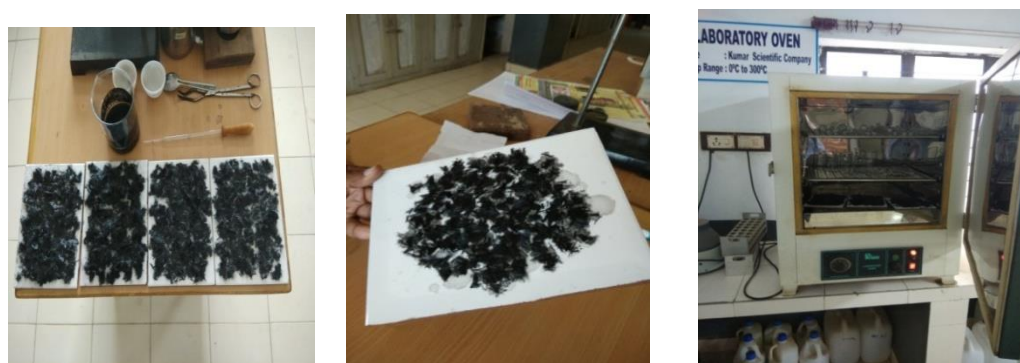
Fig 2.5 Grafting MWCNT-F on CF Surface
