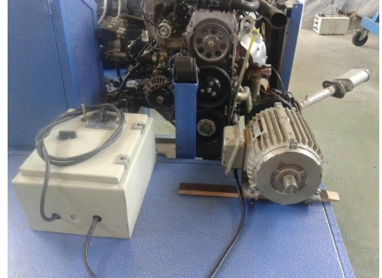
Figure 1: Motor setup, electric motor and inverter
