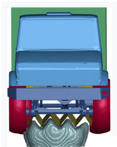
Fig. 6. Schematic view of Explosive device dispersion at 2.5ms.
