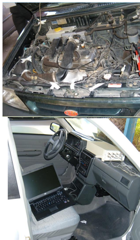
Figure 7: The data acquisition system and temperature sensors
