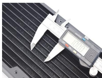
Figure 3: Radiator fin density
