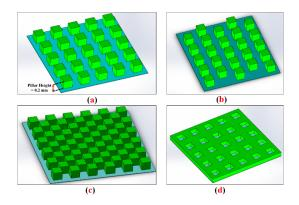
**Figure 6:** Five different examined patterns in this study: (a) a simple pattern, (b) a staggered pattern, (c) a checkered pattern, and (d) a hollow pattern. The fifth pattern was a flat (no-pillar) pattern, which is not shown. All dimensions (either all edges of cubic pillars and cubic hollows or all spaces between them) are 0.2 mm. The number of pillars and the domain size are schematic and not to scale.
