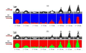
**Figure 3:** Qualitative comparison of (a) an isothermal and (b) a supercooled droplet impact between the experimental observations by [44] and the present numerical results.
