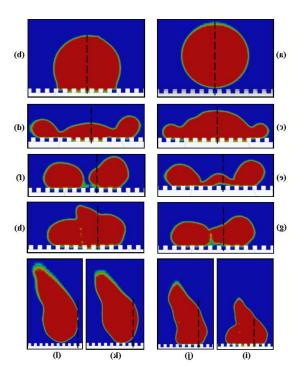
**Figure 8:** Contour of volume fraction at symmetry plane of the base simulation, the third case, at different times. (a): t = 0 ms, (b): t = 0.9 ms, (c): t = 3 ms, (d): t = 5 ms, (e): t = 6.5 ms, (f): t = 7.7 ms, (g): t = 7.8 ms, (h): t = 8.3 ms, (i): t = 9.5 ms, (j): t = 11 ms, (k): t = 12.9 ms, (l): t = 15.6 ms. The red and blue colors represent the water droplet and the air, respectively. The dashed line demonstrates the initial point of droplet impact at the beginning.
