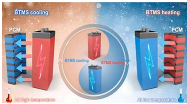
Figure 1: Principles of PCM applications in battery management systems
