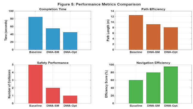
Figure 5. Comparative performance evaluation of navigation algorithms across four key metrics: (a) Task Completion Time, (b) Total Path Length, (c) Number of Collisions, and (d) Navigation Efficiency Score. The algorithms compared are the Baseline Dynamic Window Approach (DWA), DWA with Spatial Memory (DWA-SM), and the optimized DWA-SM with Bayesian Optimization (DWA-SM-Opt)
