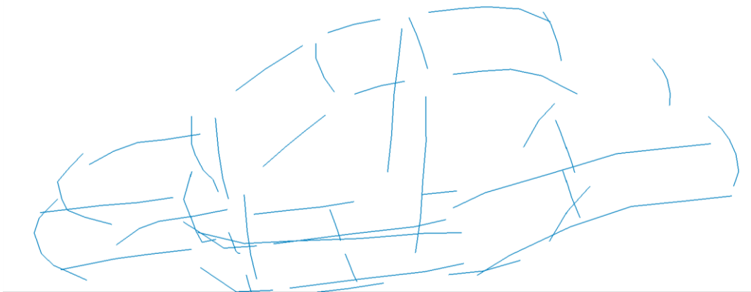
Fig3.: Equivalent beam modeling of the BIW
